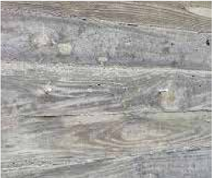
Concrete: Concrete will be used for portions of the structure, as well as exterior elements such as stairs and retaining walls. The concrete will be board formed finish in exposed exterior areas.
